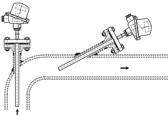
Figure 6: Classic installation of temperature sensors in piping
